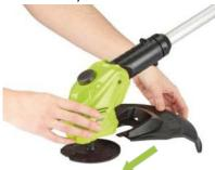
2. Connect the edge guide into its correct position on both sides of the cutting head motor.
