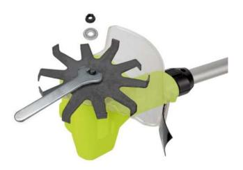
Fit the blade by inserting it on the drive axle. Insert the washer then the screw nut and secure using the wrench (supplied).
