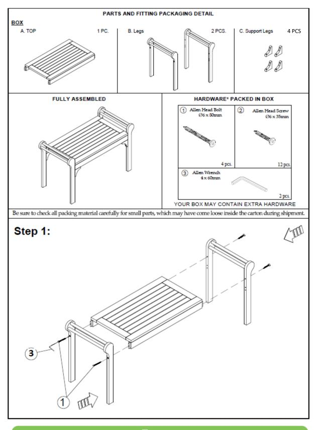
**Please Note:** Loosely attach screws and bolts when assembling. When parts are assembled, tighten the screws and bolts fully. Tightening them up immediately will often cause difficulties in assembly.
