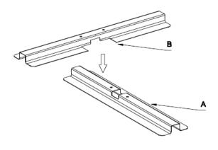
1. Join the base by placing B perpendicular on top of A.
