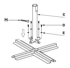
2. Place the support (C) on to the top of the base (A&B) and secure with 4x bolts (D) and washers (E).
