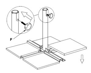
3. Loosely attach the securing bolt (F) as shown.
