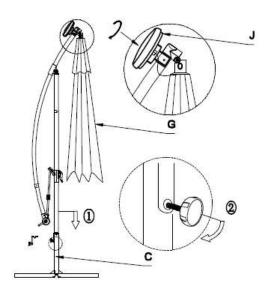
4. Attach the solar panel (J) by connecting the wire at the top of the parasol and twisting into the holder.
